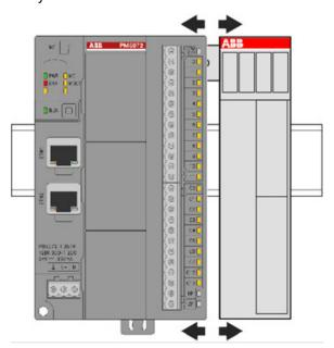
2. While pressing down I/O module pull it away from DIN rail.
