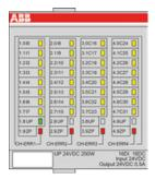
The I/O modules are the input/output unit which connects the PLC with the process. The PLC can detect controlled object data via the input interface and the data is taken as the basis for PLC control on the controlled object. In addition, the PLC sends processing results via the output interface to the controlled object to execute the control.
