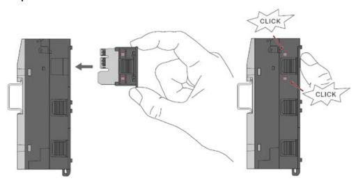
Press the option board TA51xx (or TA5300-CVR) into the slot of the processor module PM50x2 until it locks in place.
