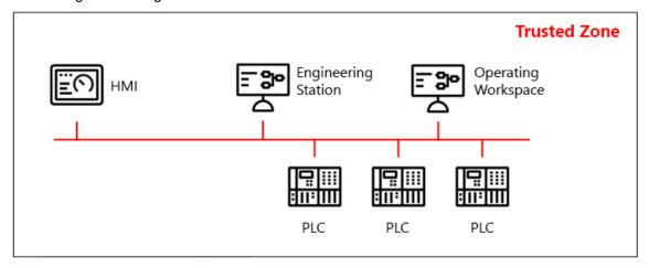
Fig. 23: Isolated automation system
