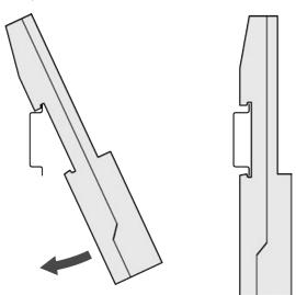
⇒ The terminal base is put on the DIN rail above and then snapped-in below.
