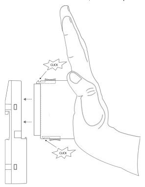
2. Press the processor module into the terminal base until it locks in place.
