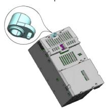
2. Fasten the processor module with two screws (diameter: 4 mm) to the metal plate.
