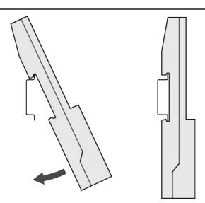
3. Demounting: A screwdriver is inserted in the indicated place to separate the terminal units.
