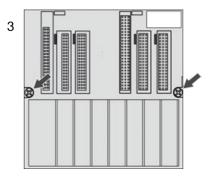
Fig. 8: Function module terminal bases, Fastening with screws
