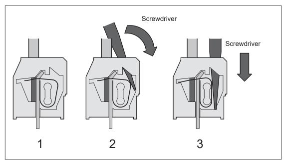
Fig. 15: Disconnect wire from the spring terminal (steps 1 ... 3)
