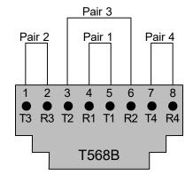
Fig. 19: Pin assignment of RJ45 sockets
