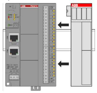
Demounting I/O modules mounted on a DIN rail
