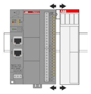
2. While pressing down processor module pull it away from DIN rail.
