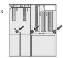
Fig. 7: Terminal bases, Fastening with screws
