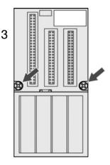
Fig. 9: Fastening with screws
