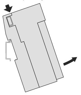
Demounting I/O modules mounted on a metal plate
