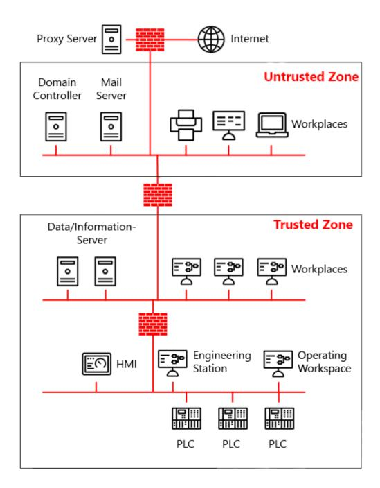
Fig. 25: Automation system and IS network
