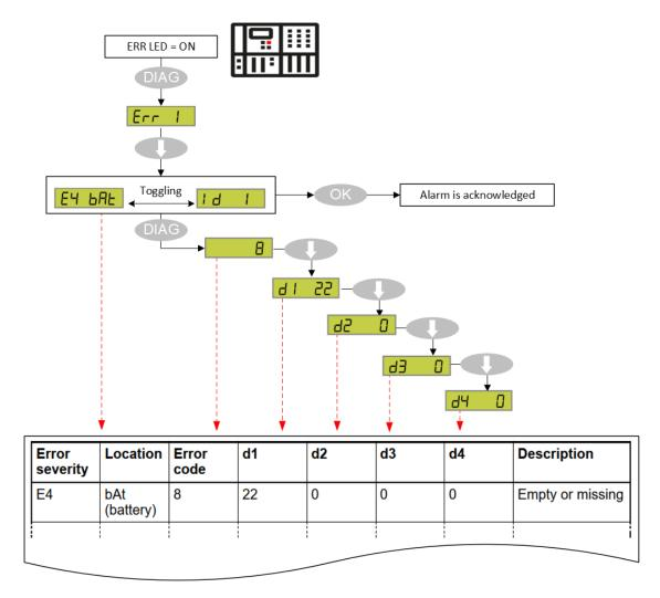
Fig. 27: Example "battery is empty or missing"
