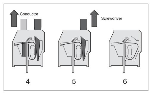
Fig. 16: Disconnect wire from the spring terminal (steps 4 ... 6)
