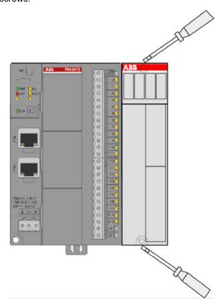
2. Remove the I/O module from the connected module by hand.
