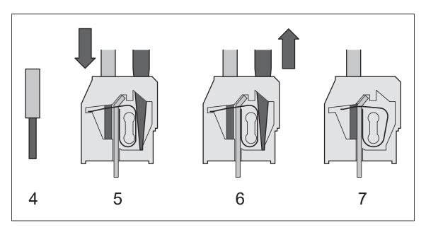
Fig. 14: Connect the wire to the spring terminal (steps 4 ... 7)
