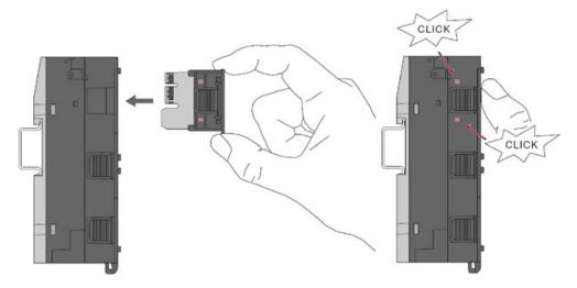
Press the option board TA51xx (or TA5300-CVR) into the slot of the processor module PM50x2 until it locks in place.
