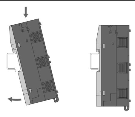
Mount the processor module at the top of the DIN rail, then snap it in below.
